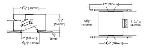
**Ceiling Cut-out** 6<sup>1</sup>/<sub>2</sub>" Dia.
