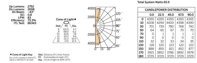
LED manufacturers maintain a tolerance of +/-7% on flux (lumens) and power (electrical) measurements.
