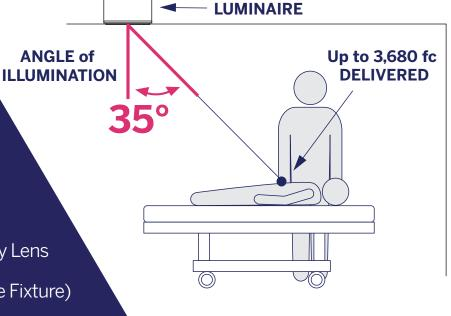
**INFRACED**® **PRO**Configurable remote-aimable lighting system for healthcare applications
