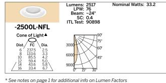
LED manufacturers maintain a tolerance of +/-7% on flux (lumens) and power (electrical) measurements.
