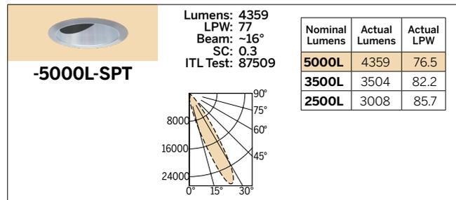
LED manufacturers maintain a tolerance of +/-7% on flux (lumens) and power (electrical) measurements.
