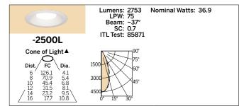
▲ Cone of Light Key Dia. (in ft.) shown is where FC value is half the FC at nadir. Dist. Distance (Ft.) from fixture FC Footcandles at nadir (0°) Dia. Circle of light at 50% of FC
