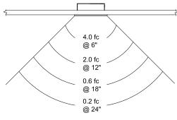
\* Based on 14" mounting height; measuring footcandles at the floor perpendicular to the lens.
