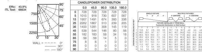
Photometry based on: 6200 lumens - 70W 3400 lumens - 39W
