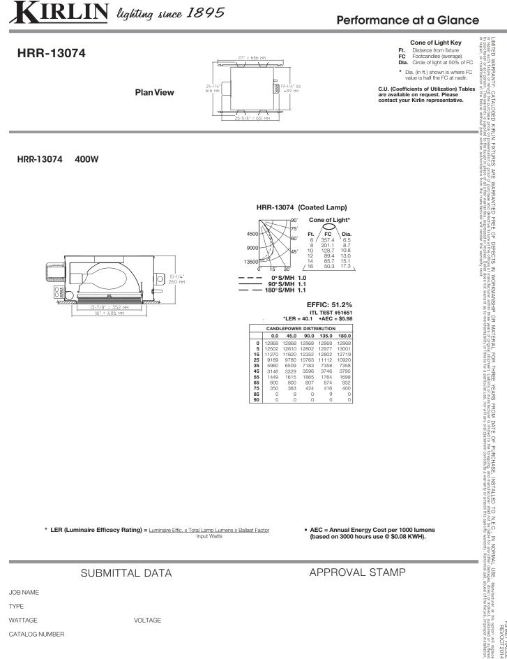
\* LER (Luminaire Efficacy Rating) = Luminaire Effic. x Total Lamp Lumens x Ballast Factor Input Watts
