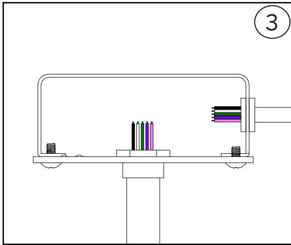
Connect the line (black), neutral (white), DIM+ (violet), and DIM- (pink) wires to the corresponding incoming power and control wires using wire nuts (supplied by others).
