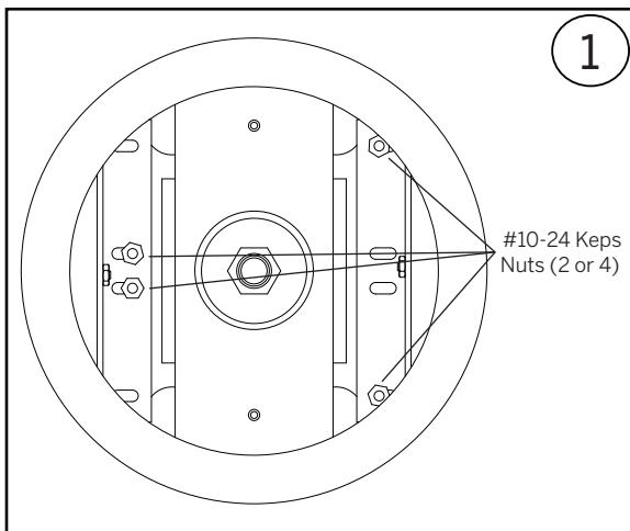
For driver service, continue from the previous service steps. Remove the #10-24 keps nuts (2 or 4) to remove the driver bracket(s) (1 or 2).
