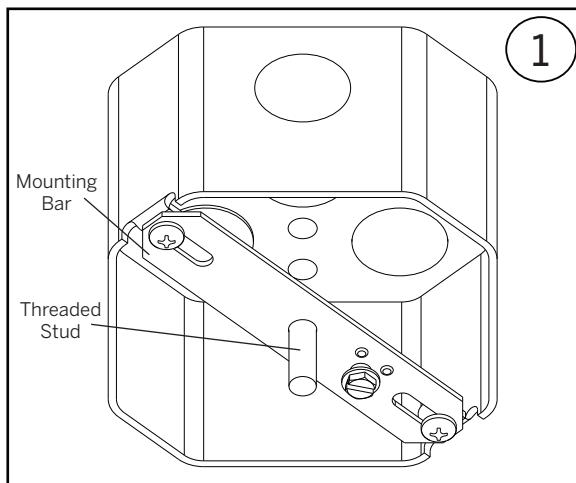
Insert the supplied 1/4"-20 x 1" threaded stud into the mounting bar.
