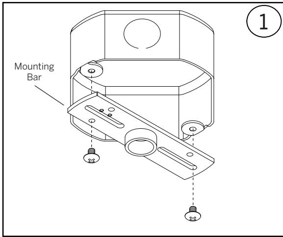
For pendant and cable mount installations, install the supplied mounting bar to the octagonal junction box (supplied by others) using junction box hardware (supplied by others).
