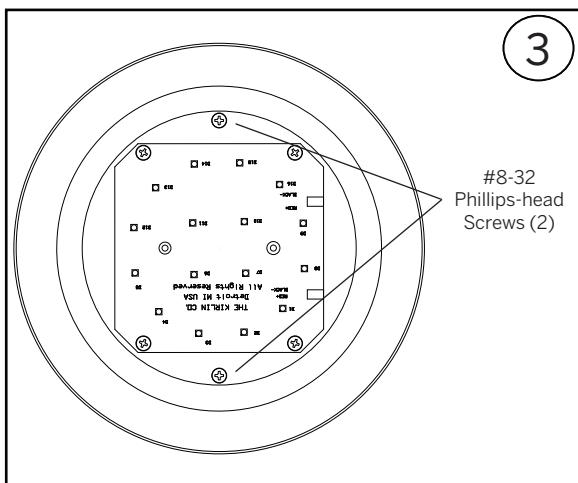
Remove the #8-32 Phillips-head screws (2) and disconnect any wire connections to remove the LED board assembly. Repeat these steps in reverse for reinstallation.
