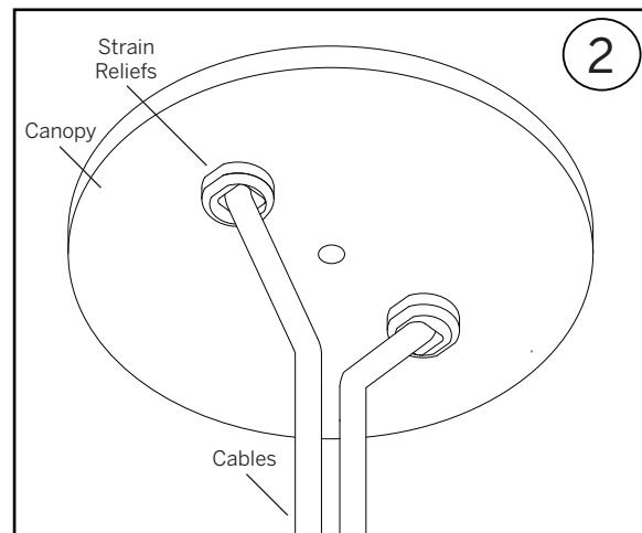
Insert the supplied cables through the supplied canopy, securing using the supplied strain reliefs.
