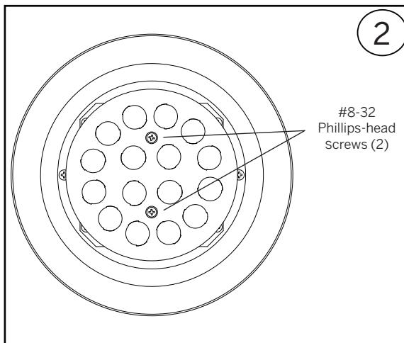
Remove the #8-32 Phillips-head screws (2) to remove the LED optic assembly.
