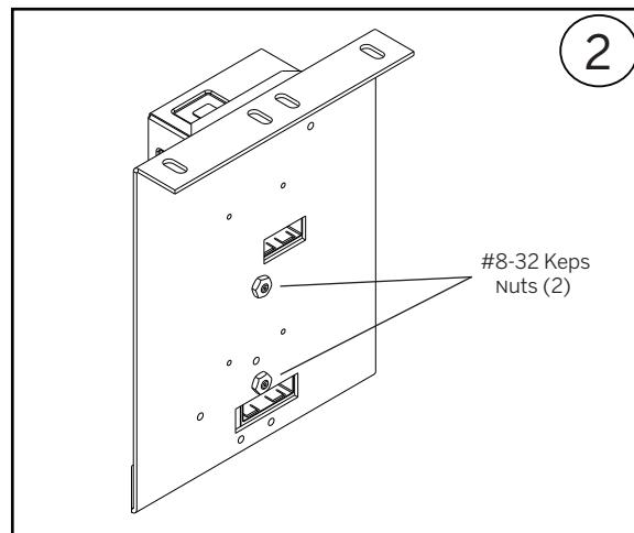
Remove the #8-32 keps nuts (2) to remove the driver from the driver bracket. Make note of and disconnect any connections where necessary. Repeat these steps in reverse order for reinstallation.
