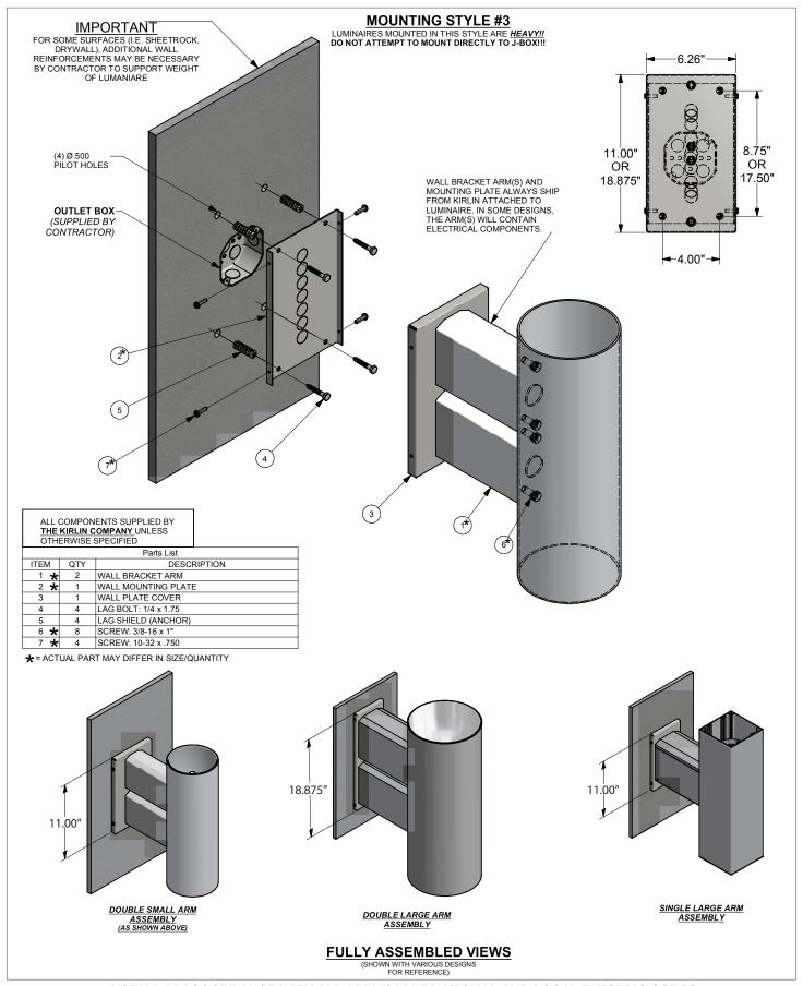
INSTALL IN ACCORDANCE WITH ALL APPLICABLE NATIONAL AND LOCAL ELECTRIC CODES INSTALL IN ACCORDANCE WITH ALL MARKINGS APPEARING ON OR INSIDE LUMINAIRES FOR OUTDOOR INSTALLATIONS, USE SILICONE TO CAULK AROUND ALL EXPOSED SEAMS
