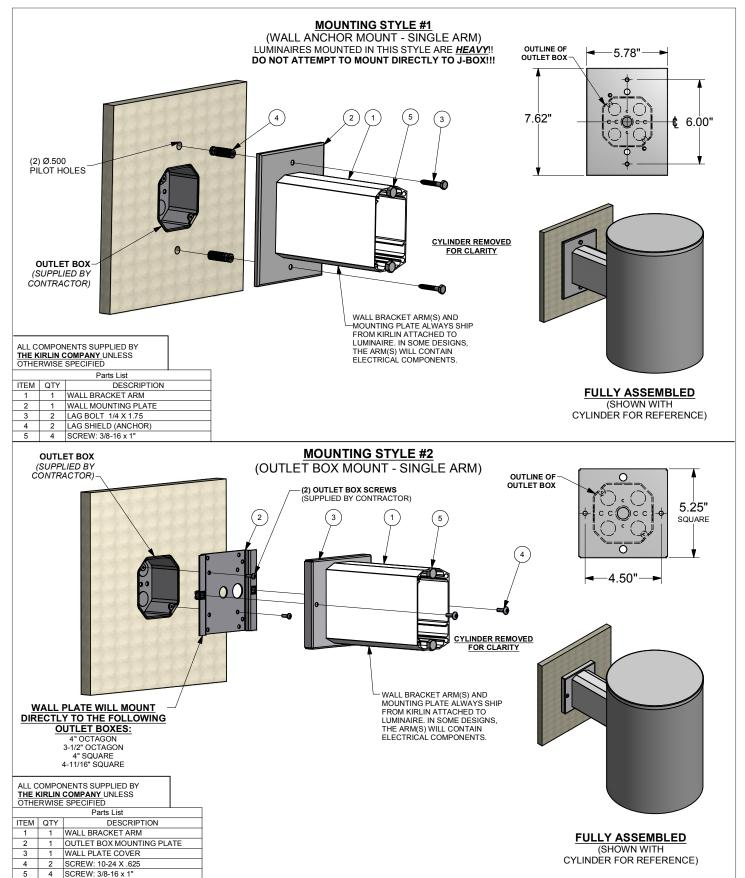
INSTALL IN ACCORDANCE WITH ALL APPLICABLE NATIONAL AND LOCAL ELECTRIC CODES INSTALL IN ACCORDANCE WITH ALL MARKINGS APPEARING ON OR INSIDE LUMINAIRES FOR OUTDOOR INSTALLATIONS, USE SILICONE TO CAULK AROUND ALL EXPOSED SEAMS
