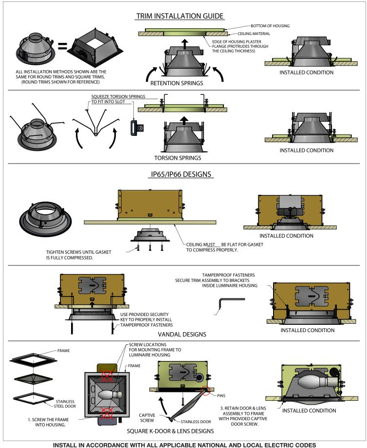
INSTALL IN ACCORDANCE WITH ALL MARKINGS APPEARING ON OR INSIDE LUMINAIRES
