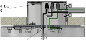
ROUTE LUMINAIRE WIRES & SAFETY CABLE THRU CENTER HOLE & INTO OUTLET BOX.
